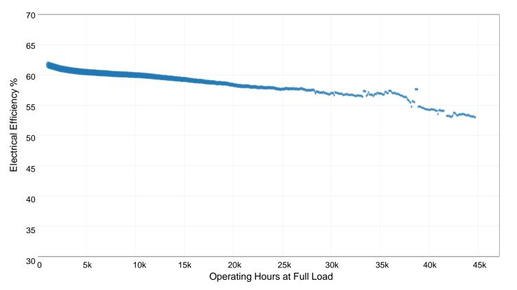
Data is composite of commercial operating BG-0 units at Full Power output over 5 years.
